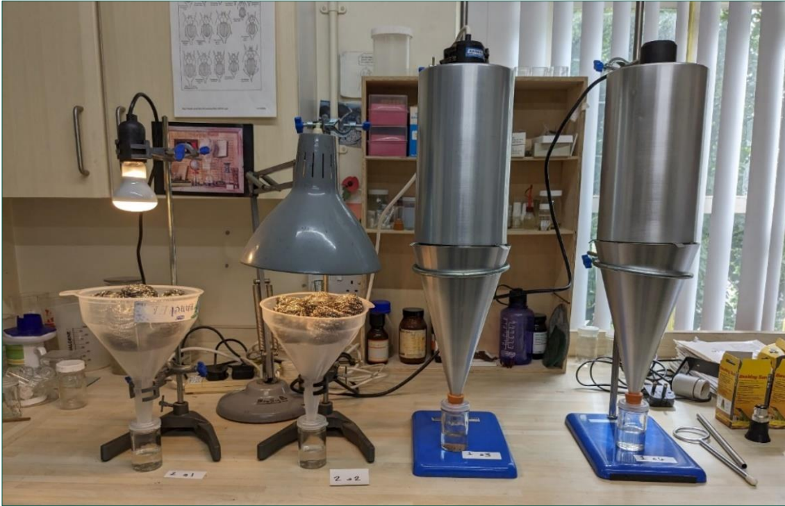
Figure 6. Tullgren funnel extraction setup.
